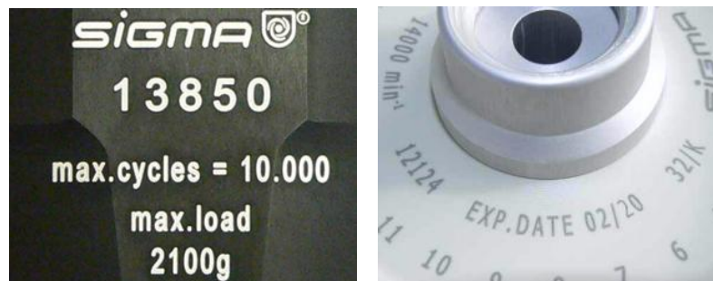
Fig. 4: Different service life – engraving on the bucket/rotor
